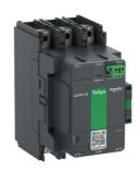
High power contactor, TeSys Giga, 3 pole (3NO), AC-3 <=440V 115A, standard version, 48...130V wide band AC/DC coil
